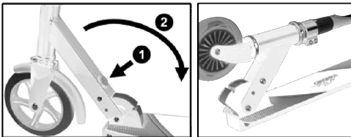
The front wheel and handlebar assembly is hinged at the front of the deck. To open the scooter into its riding position, simply press the red button and lift the handlebar column up. When the handlebars and front wheel assembly are in the correct riding position, the folding mechanism will snap and lock. To fold the scooter flat, press the button again and move the column downwards, until the locking mechanism snaps.
